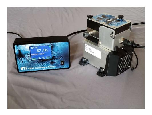
Chilled mirror condensation dewpoint hygrometers provide precise, stable and repeatable, standards grade measurement of humidity in an industrial or laboratory environment. The chilled mirror measurement is a fundamental physical measurement of humidity, it is not based on the humidity absorption properties of plastics or other humidity sensing materials. It is only dependent on the physical properties of water and accurate temperature measurement.
